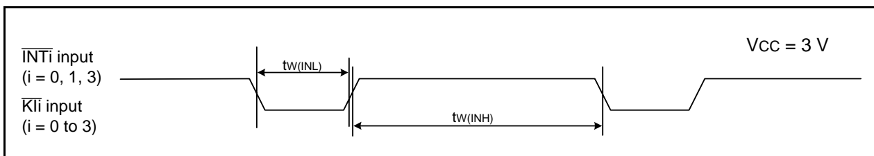
Figure 5.15 Input Timing for External Interrupt \overline{INTi} and Key Input Interrupt \overline{Kli} when Vcc = 3 V
